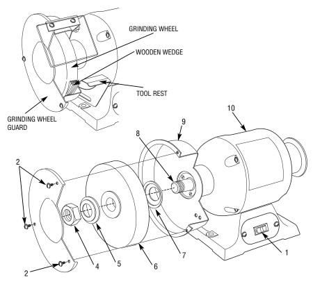
FIGURE 4. REPLACING GRINDING WHEEL
